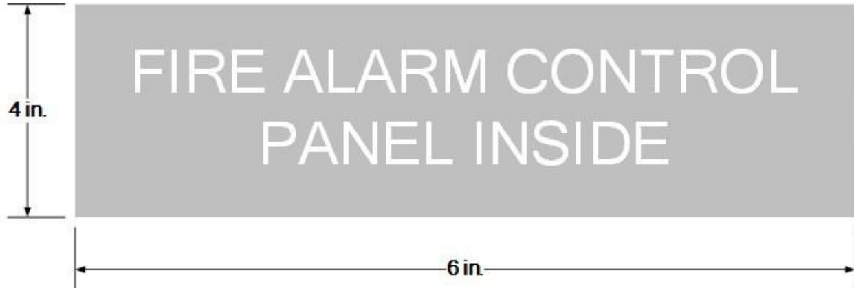
FIGURE F-5.2: FIRE ALARM CONTROL PANEL SIGNAGE
